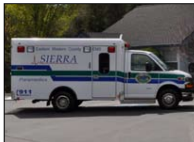
A unique feature of the Crestline ambulances are the powder coated aluminum body.
